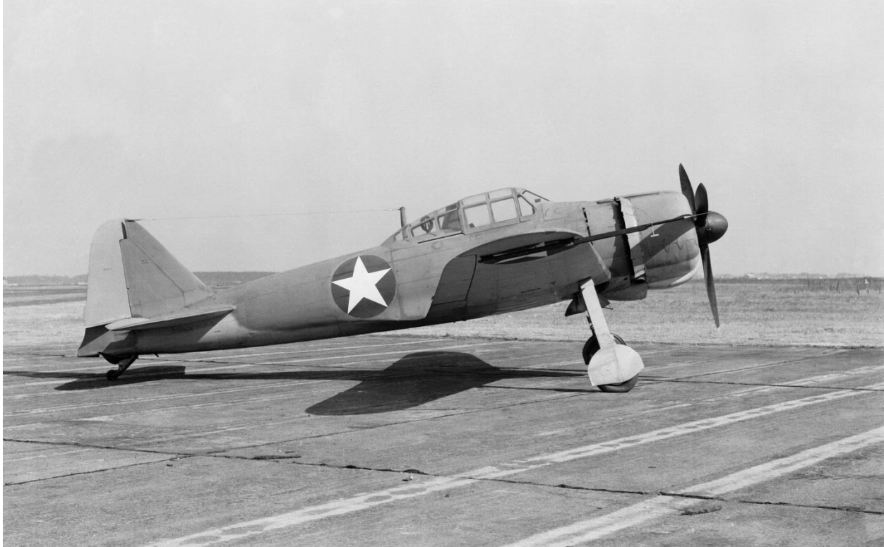
Japanese Mitsubishi Zero on the NACA Langley Memorial Aeronautical flight line on March 8, 1943. The aircraft had been repainted in U.S. Navy colors and insignia but retained its Japanese serial number “4593” barely visible on the vertical tail. Koga’s Zero was unique in having a short stubby wooden radio mast. Aircraft is shown after installation of NACA wing-tip boom for flight tests at Anacostia NAS.
