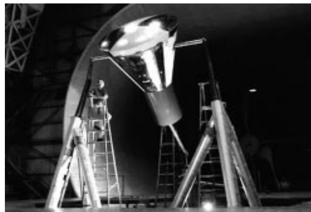
NASA Langley Research Center photo #59-336 A full-scale model of the Mercury capsule being tested in the NASA Langley 30- by 60-Foot Full-Scale Wind Tunnel.
