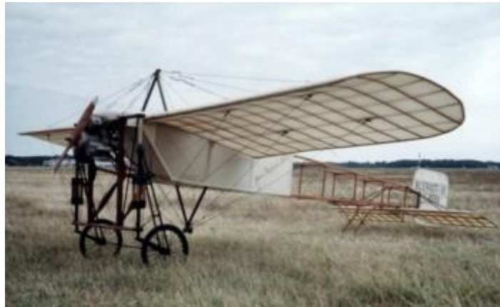
The flying wires can be seen in this photo of a Blériot
